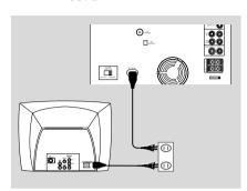
After everything is connected properly, plug in the AC power cord to the power outlet.
